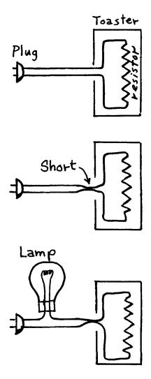
the toaster's resistor it still has to go through the light bulb's resistor. And the bulb's resistance stops the current from running wild. Of course, the light bulb hinders the flow of current through the toaster and will not let it get as hot as normal, but it saves the fuse.
