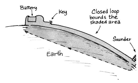
transatlantic cable was so long that small currents could flow back and forth in it even with the key open! Current just swished back and forth around the open loop, piling up at the ends. The length of the cable provided an electric storage capacity, the capacitance, which made the pile-up possible. This was a fascinating discovery at that time. The construction of the transatlantic cable was the "moon project" of its day.
