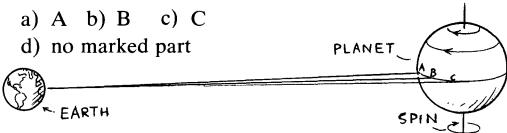
Objects are detected by radar, that is, by sending out radio signals and then receiving the radio waves reflected back from the objects. In the sketch we see that a radar signal is sent from earth to a planet. The signal from which part of the planet returns to the earth first?
