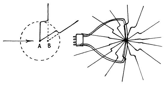
Because the x-rays go off to the sides, x-ray tubes are designed to have x-rays come out of them on the side. The thing that stops the electrons is called the target. The target is slightly tipped to enhance the sending of x-rays off to one side. (The reason the electrons rush to the
