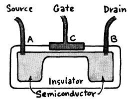
Were the bridge made of copper this electric valve wouldn't work because the top of the bridge would get positive enough to shield the material below it from the negative charge on the gate. But in a semiconductor there are not enough free electrons to make the top of the bridge sufficiently positive to shield itself.
