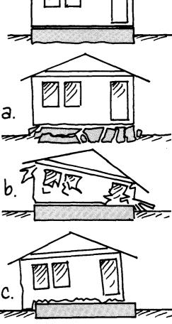
Many houses consist of a wooden frame structure that simply rests upon a concrete foundation or slab. In the event of a moderately severe
