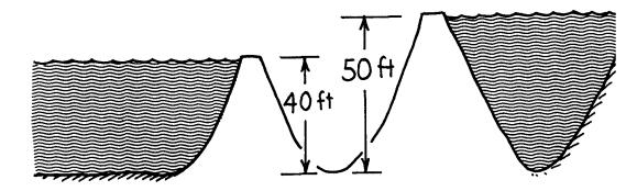
Dams are constructed thicker at the bottom than at the top because water pressure against the dam increases with depth. But how about the volume of water held back by a dam?
