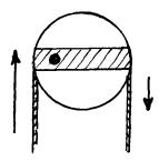
The crazy pulley is called an *eccentric* pulley. Can you see how the eccentric pulley allows the compound bow to be held in the cocked position with very little tension in the bow string? And can you see that unlike the conventional bow, the tension increases as the arrow is shot?
