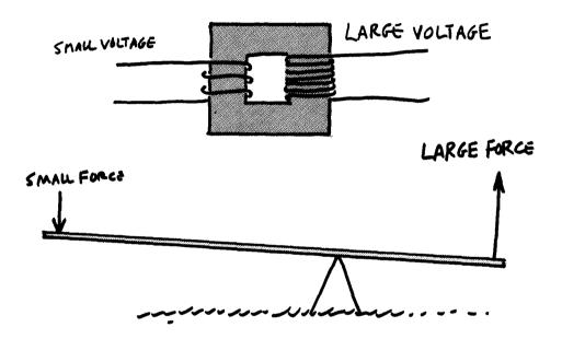
A transformer is very much like a lever. The power that comes out of one end of a lever is equal to the power that goes into the other, because a lever is not a source of power. The lever can convert a small, rapidly moving force to a large, slowly moving force, or vice versa. Similarly, a transformer can convert a small voltage motivating a large electric current into a large voltage motivating a small electric current, or vice versa.
