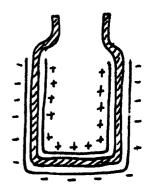
could lie together in the same bed provided an upright board prevented any touching. In a Leyden Jar, opposite charges are prevented from touching by means of the glass bottle. Suppose the inside is charged + and the outside -. Then electric force field lines run from the + charges on the inside foil to the -
