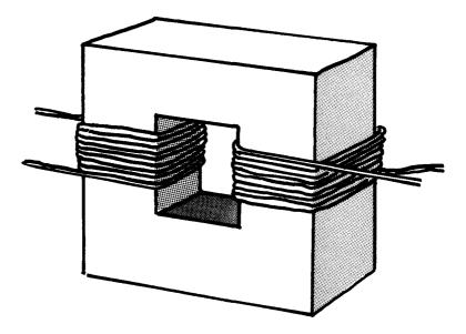
magnet which "generates" current in the output or secondary coil. Into a perfect transformer is fed a particular voltage and current, hence a particular power (wattage). Out of the transformer must come the same
