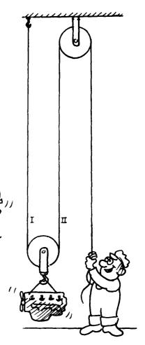
weight of the kid need only be one third the weight of the man. Similarly, to lift the engine one meter, the mechanic must pull two meters of rope — one meter from Line I and one meter from Line II — so the mechanic pulls with a force that is only half the weight of the motor.
