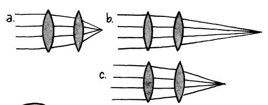
Most pocket magnifiers have two lenses which can be used one at a time or together when a stronger lens is required.
