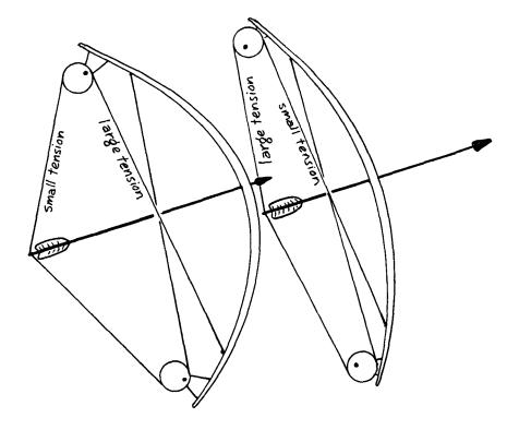
Incidently, mechanical engineers have a name for this kind of variable leverage mechanism. It is called a *toggle* action. Many electric light switches have toggle action, whence the name *toggle switch*.
