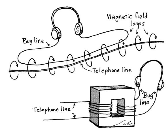
We can think of the telephone wire as the primary and the bug line as the secondary of a transformer. The bug will work even better if, like a transformer, the wires are wrapped around a hunk of iron.
