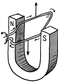
Underlying electric meters and motors is the simple fact that electric current is deflected in a magnetic field. The deflecting force is always perpendicular to both the current and the magnetic field as shown in the sketch.
