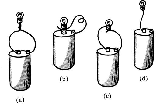
A simple electric circuit can be made with a dry cell, a lamp, and some wire. In which of the arrangements shown will be lamp be lit?
